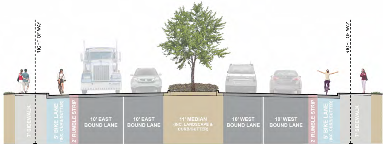
SECTION 'A' Alternate - Buffered One Way Bike Lane Each Direction w/ Landscape Median
