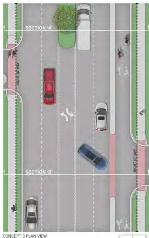
SECTION 'A' - Protected Two Way Bike Lane w/ Landscape Median
