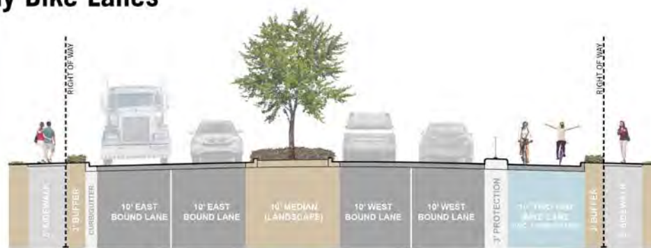
SECTION 'A' - Protected Two Way Bike Lane w/ Landscape Median
