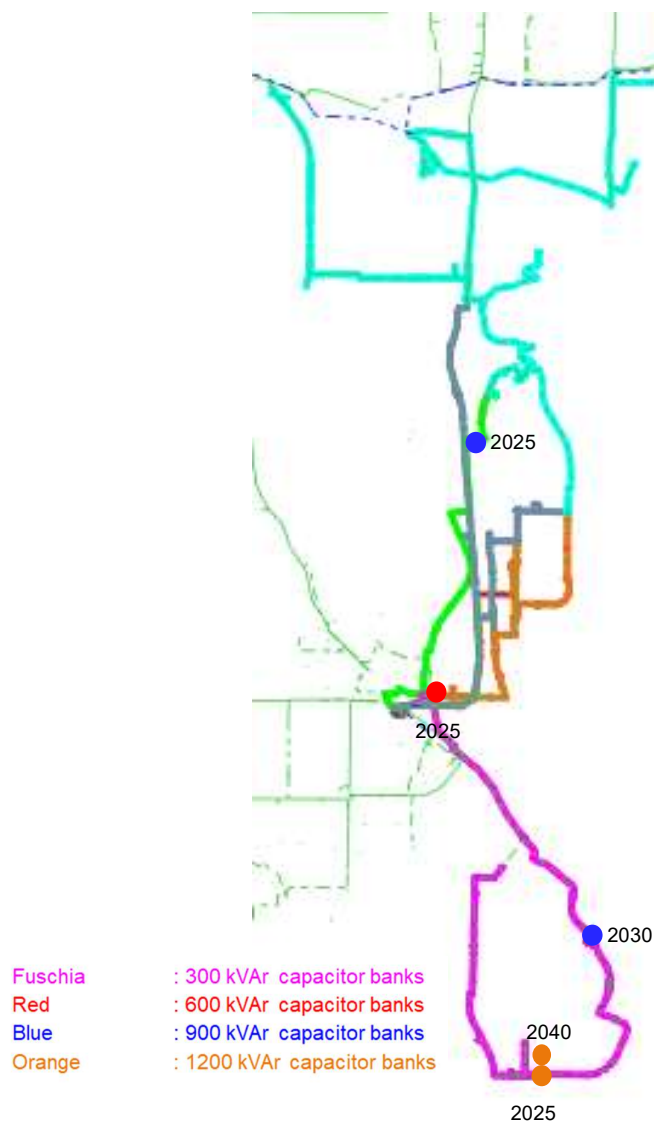
Figure 5-91 New capacitor banks in Area 11
