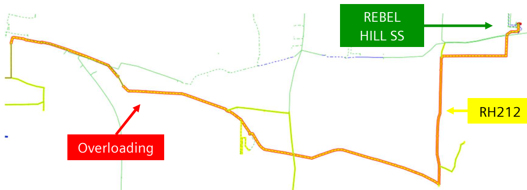
Figure 5-82 Overloading violation under GS232 emergency condition in 2025
