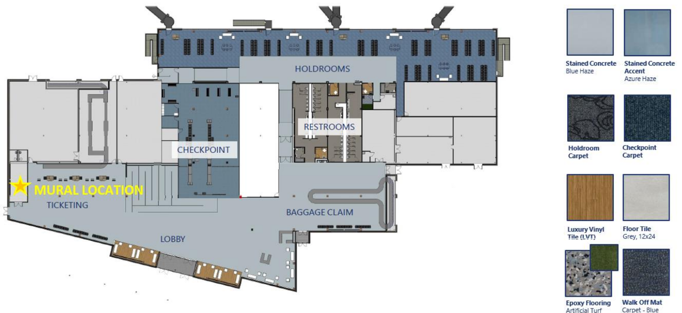
Terminal Floor Plan and Building Materials
