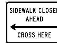
R9-11L "SIDEWALK CLOSED AHEAD" SIGN
