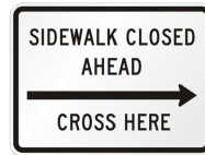
R9-11R "SIDEWALK CLOSED AHEAD" SIGN
