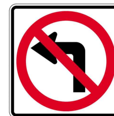
R3-2 "NO LEFT TURN" SIGN
