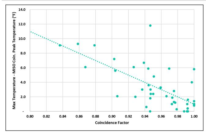
As maximum temperature deviates from MISO system peak-producing temperatures, CMWL's coincidence factor declines.
