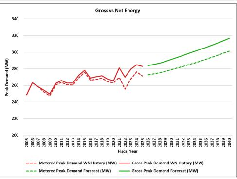
Separation between net and gross energy driven by Truman solar and net-metering solar growth.
