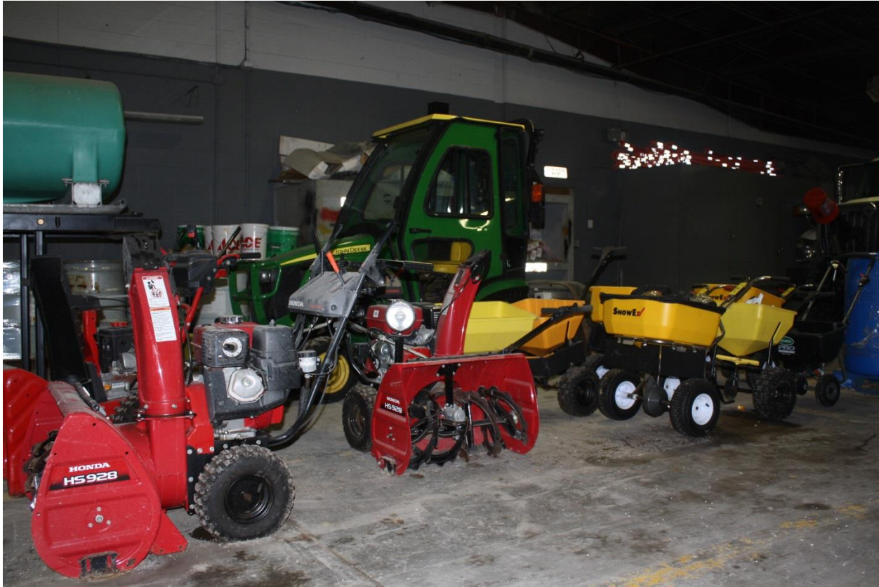
Figure 18 Snow blowers, salt buggies and garden tractor for sidewalk and pedway snow and ice control
