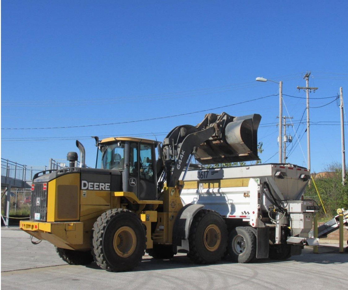
Figure 5 Loading spreader at salt storage facility
