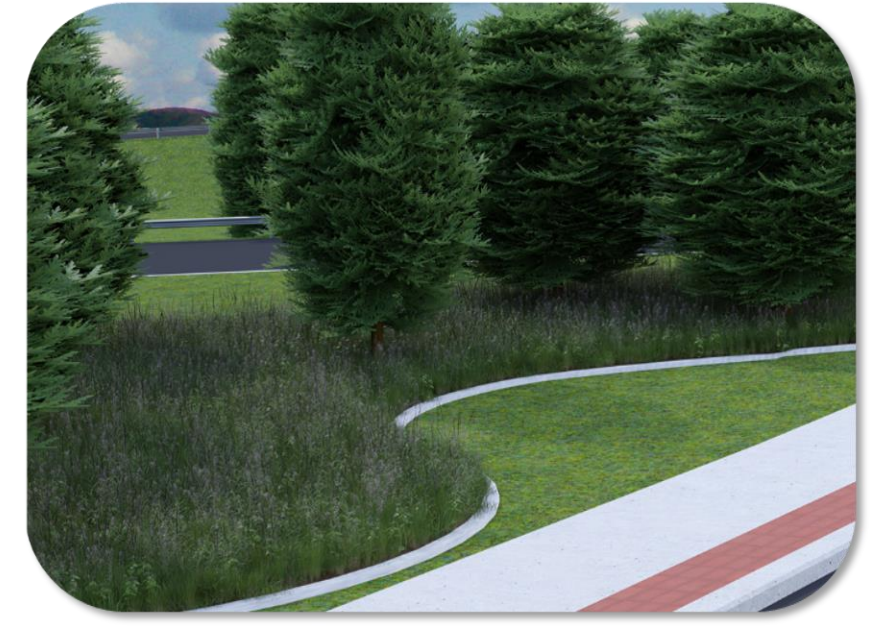
Concrete Planter Curb
