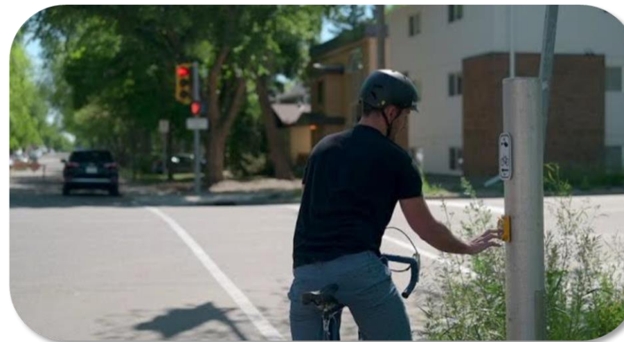
Example of pushbutton location for cyclist
