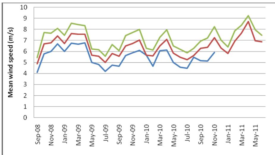
The green line represents observations at 147 meters, the red line is for 98 meters, and the blue line shows the measurements at 68 meters.
