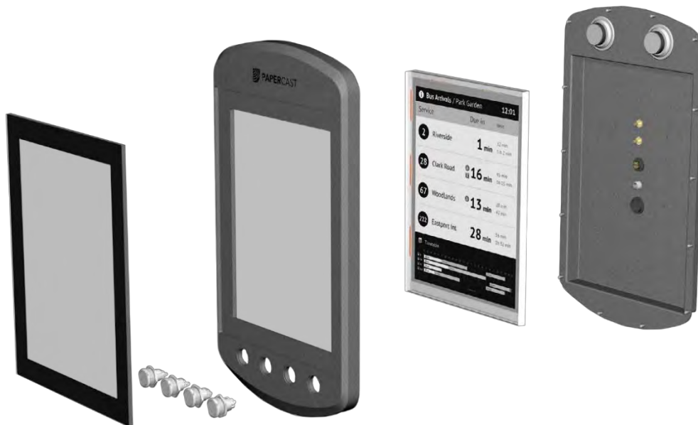
Figure 62: Detail view of the anti-theft assembly and unit construction.
