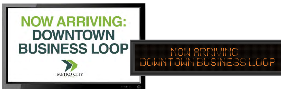
Figure 53: SPOT's AVA system determines which media to deploy based on the type of announcement systems present at an individual station or vehicle.
