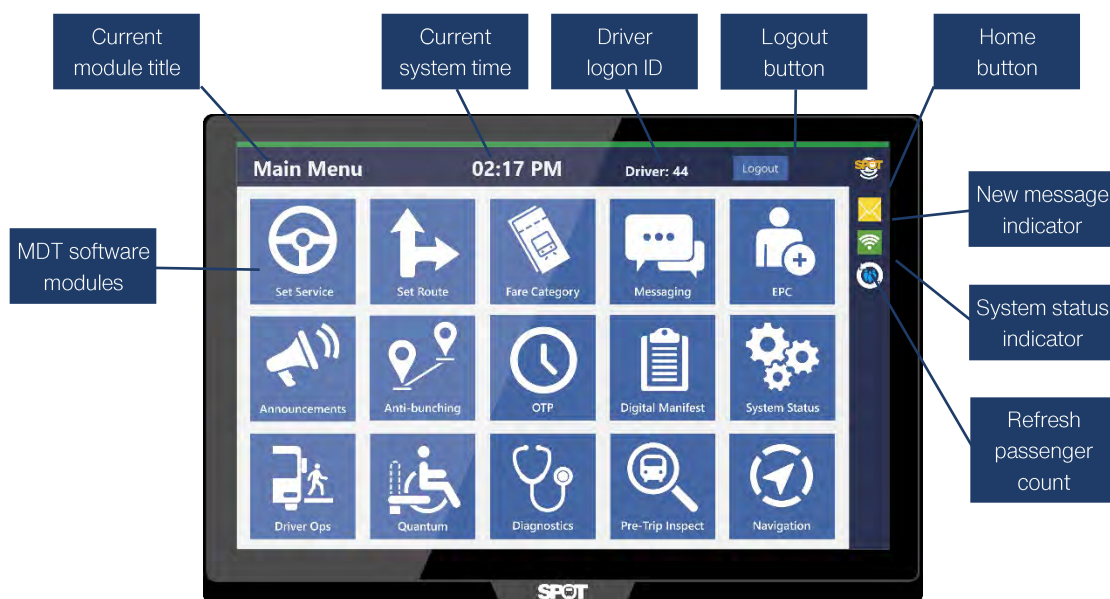
Figure 9: The MDT main menu provides the driver with easy one-touch access to all installed software modules.
