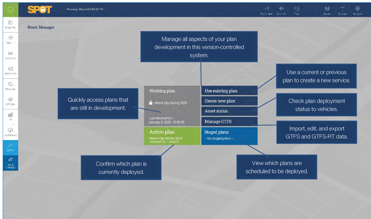
Figure 22: The Route Manager home screen provides a quick launch point for a variety of plan-related tasks.
