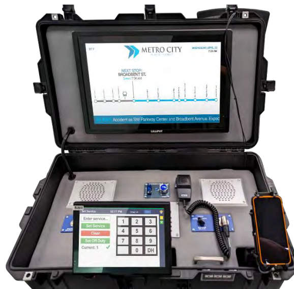
Figure 66 Bus in box - Portable training aid for on-board bus technologies
