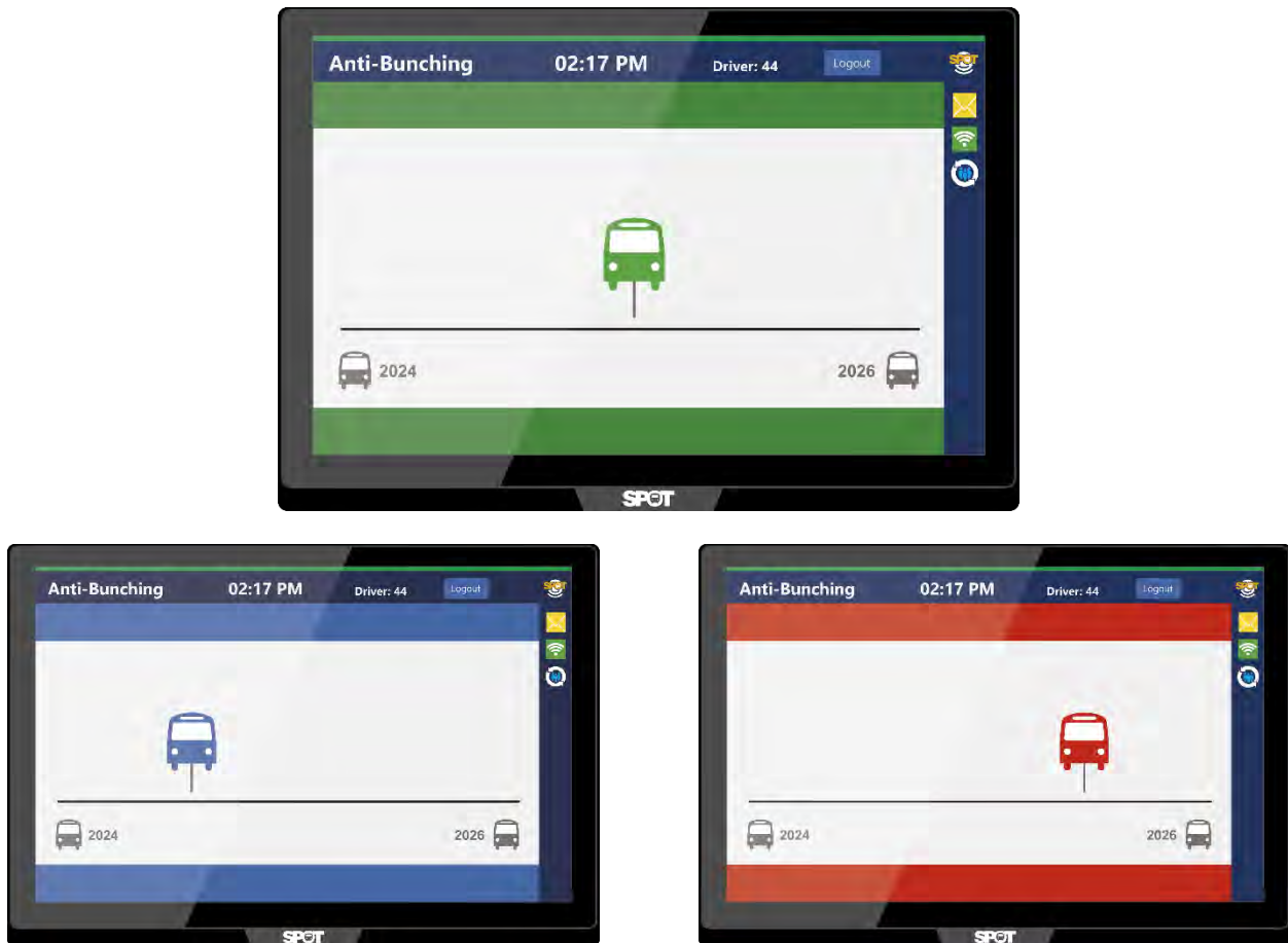
Figure 19: Vehicle position and spacing display in easy-to-understand color codes. Green represents the optimal spacing between assets on the same route; blue indicates a driver is too far away from the vehicle in front, and red shows the bus/shuttle is too close to the one in front.
