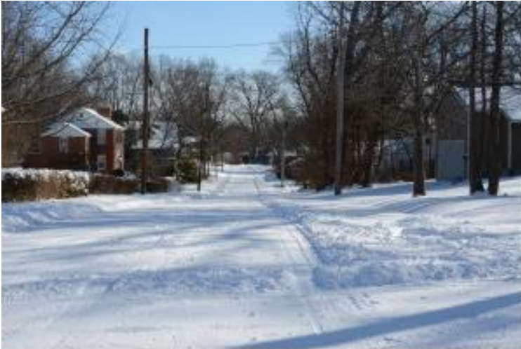
This is a city street showing both driving lanes as plowed yet no pavement visible. This road meets the definition of passable.
