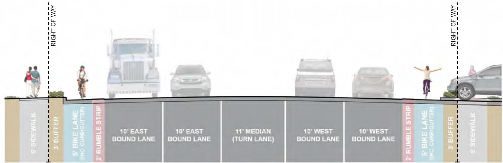
SECTION 'B' - Buffered One Way Bike Lane Each Direction @ Curb Cut w/ Turn Lane
