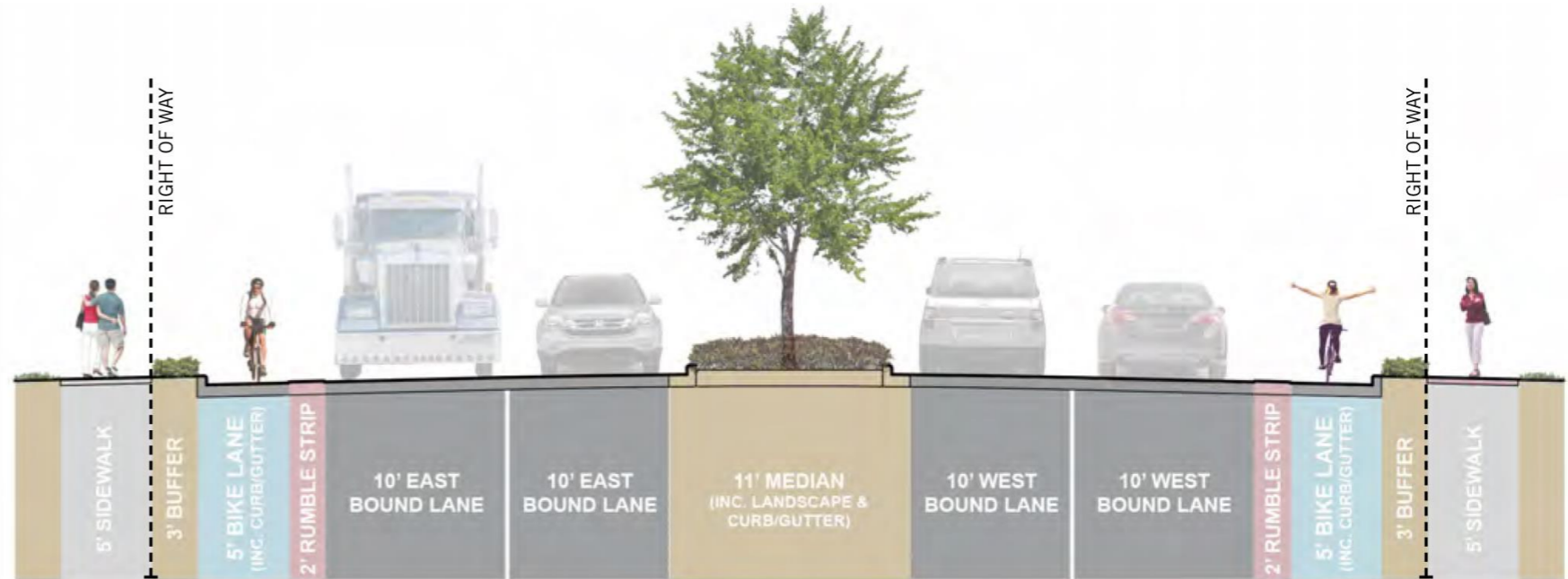
SECTION 'A' - Buffered One Way Bike Lane Each Direction w/ Landscape Median
