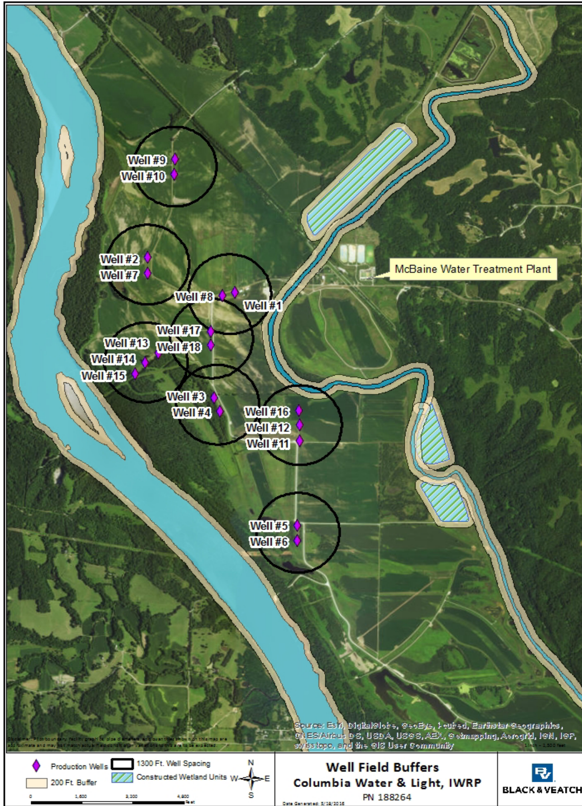
Figure 5-1 Existing well field with surface water and well field spacing buffers applied.
