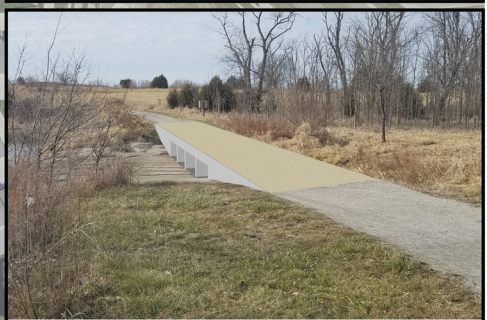
EXISTING LOW WATER CROSSING PROPOSED LOW WATER CROSSING 16 feet wide to provide a 8 foot wide trail with 4 foot wide shoulders and curbing Approximately 60 feet long
