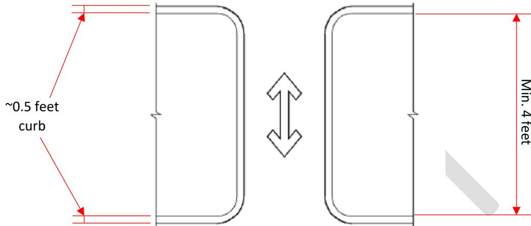
**Figure 11: Island cut through**<sup>61</sup>
