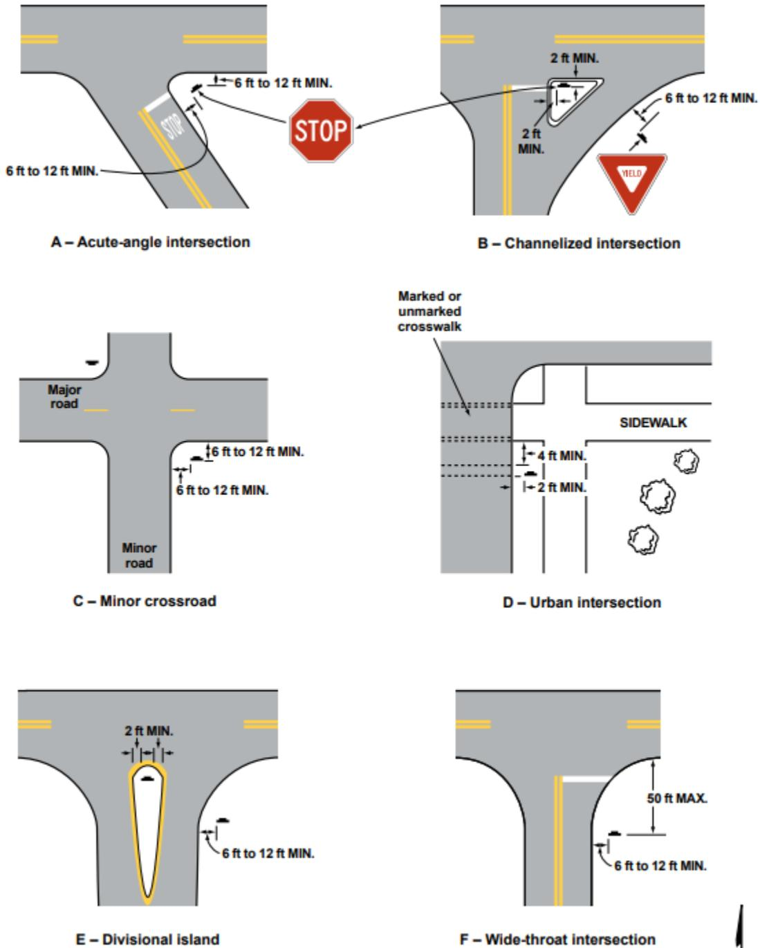
Note: Lateral offset is a minimum of 6 feet measured from the edge of the shoulder, or 12 feet measured from the edge of the traveled way. See Section 2A.16 for lower minimums that may be used in urban areas, or where lateral offset space is limited.
