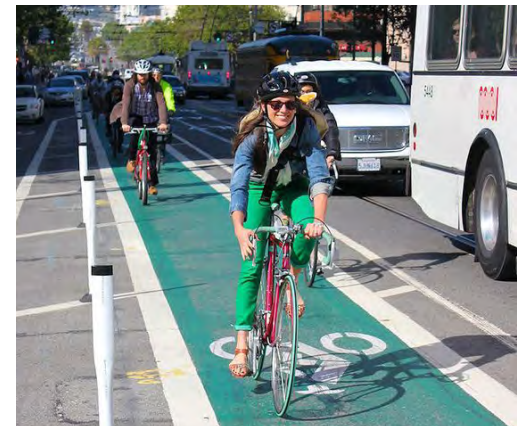
Precedent: Bike Lane with Painted Separator Strip
