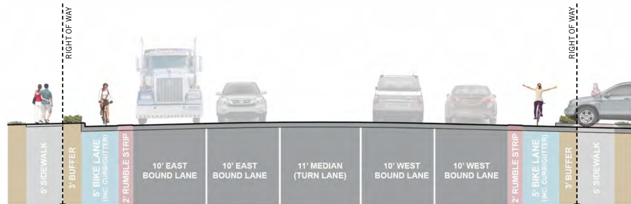
SECTION 'B' - Buffered One Way Bike Lane Each Direction @ Curb Cut w/ Turn Lane
