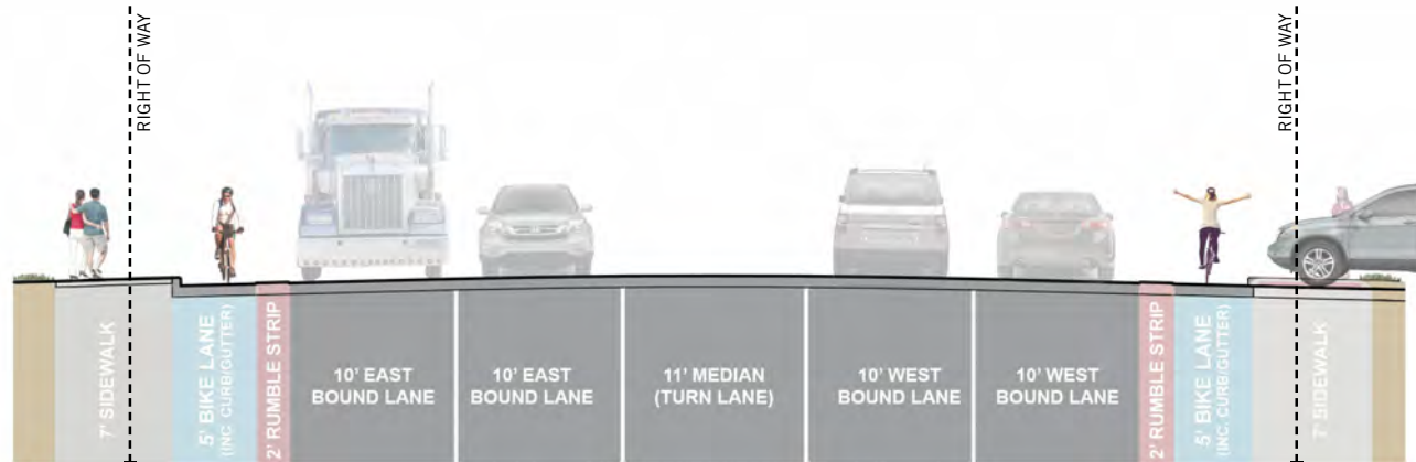
SECTION 'B' Alternate - Buffered One Way Bike Lane Each Direction @ Curb Cut w/ Turn Lane
