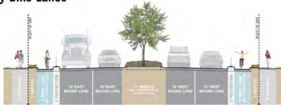
SECTION 'A' - Protected One Way Bike Lane Each Direction w/ Landscape Median
