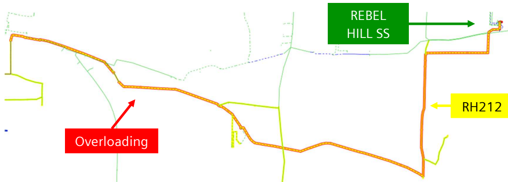
Figure 5-82 Overloading violation under GS232 emergency condition in 2025
