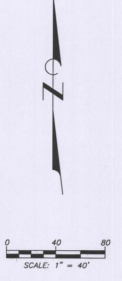
BEARINGS ARE REFERENCED TO MISSOURI STATE PLANE COORDINATE SYSTEM (NAD 1983) CENTRAL ZONE.
