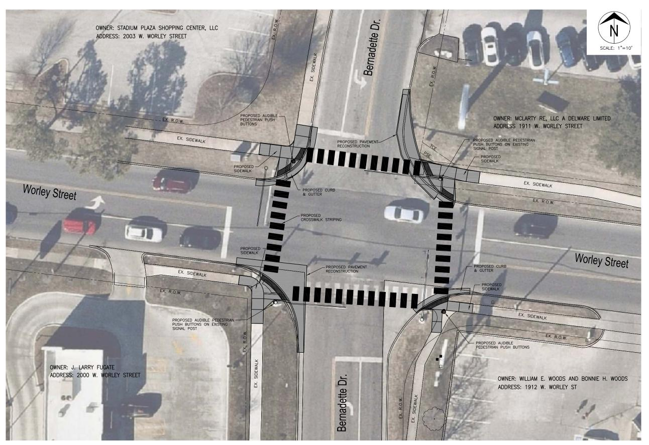
AUDIBLE PEDESTRIN SIGNALS, SIDEWALKS & STRIPING PLAN
