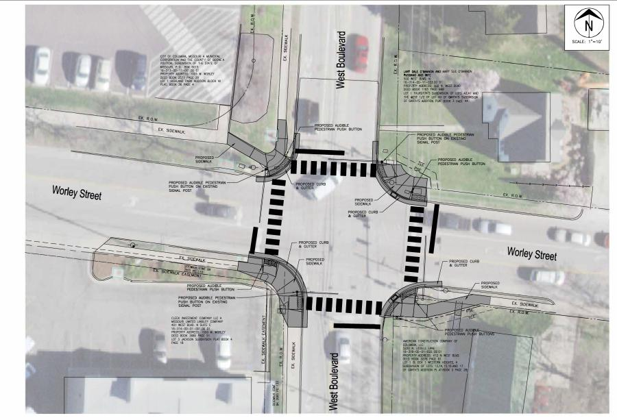
AUDIBLE PEDESTRIAN SIGNALS, SIDEWALKS & STRIPING PLAN
