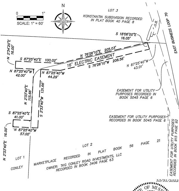
BEARINGS ARE REFERENCED TO MISSOURI STATE PLANE COORDINATE SYSTEM (NAD 1983) CENTRAL ZONE.
