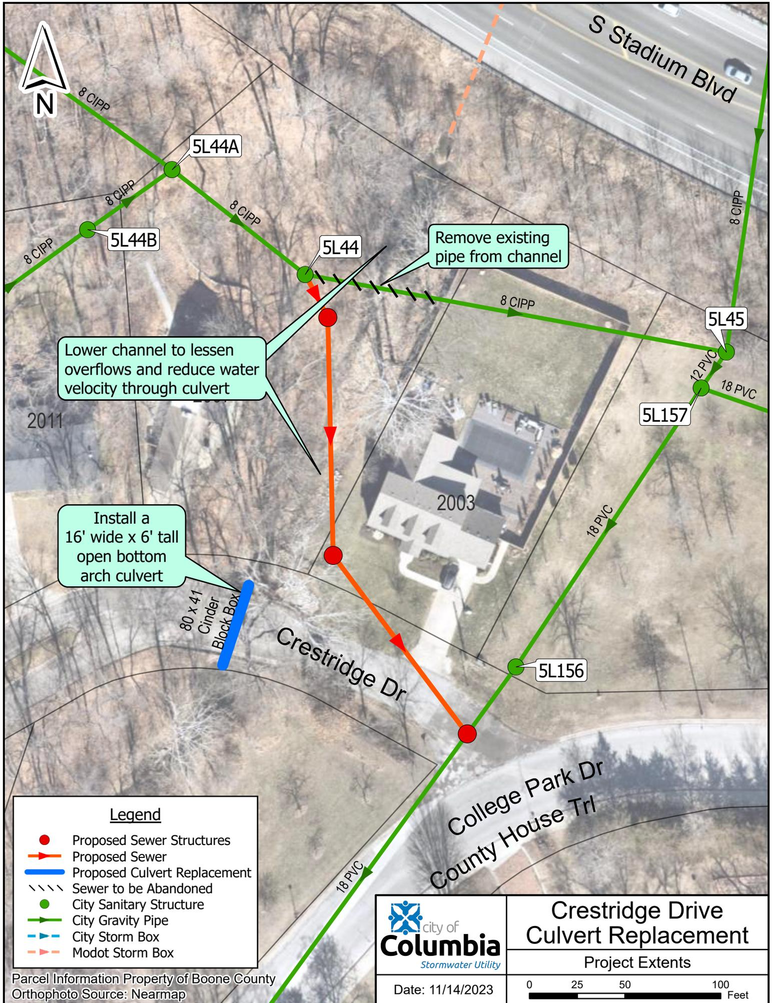
Lower channel to lessen overflows and reduce water velocity through culvert
