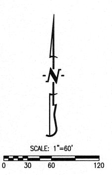
BEARINGS ARE REFERENCED TO GRID NORTH OF THE MISSOURI STATE PLANE COORDINATE SYSTEM (CENTRAL ZONE) OBTAINED FROM GPS OBSERVATION.
