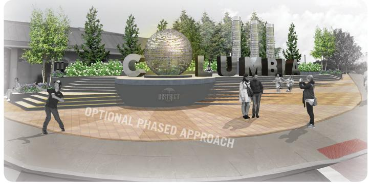
**GATEWAY PLAZA: PHASE TWO** Phase <u>two</u> elements would include: -Heritage Columns -Plaza Pavement -Interpretive Plaques -Steps and retaining walls Estimated Cost Phase Two: \$2,125,000
