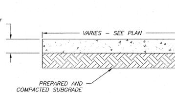
1. CONCRETE SIDEWALK TO HAVE 1.0% (2.0% MAX.) CROSS SLOPE UNLESS OTHERWISE SHOWN. 2. EXPANSION JOINTS ARE TO BE SET EVERY 100' WITH 1/2" EXPANSION MATERIAL AND BE FLUSH WITH THE TOP OF THE WALK. 3. TRANSVERSE SAW CUT JOINTS AT SPACING EQUAL TO
