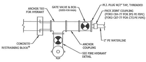
IF FIRE HYDRANT IS NOT REQUIRED, THEN ANCHOR CONCRETE RESTRAINING BLOCK TO GATE VALVE AND OMIT ANCHOR COUPLING
