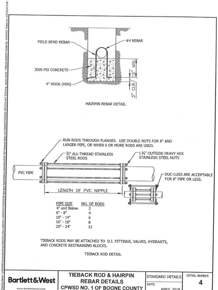
TIEBACK RODS MAY BE ATTACHED TO D.I. FITTINGS, VALVES, HYDRANTS, AND CONCRETE RESTRAINING BLOCKS.
