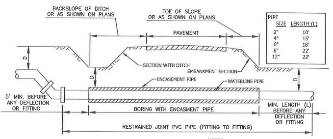
"D"- 48" FOR STEEL ENCASEMENT AND 72" FOR HDPE ENCASEMENT UNLESS OTHERWISE **SPECIFIED**
