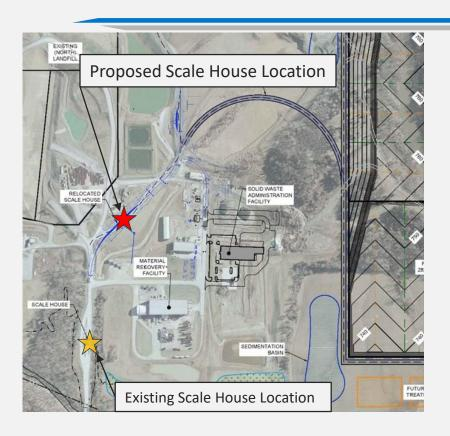
Site grading, road construction, new scale house, relocating two existing scales, two new scales, vehicle wheel wash system, security cameras and demolish existing scale house.
