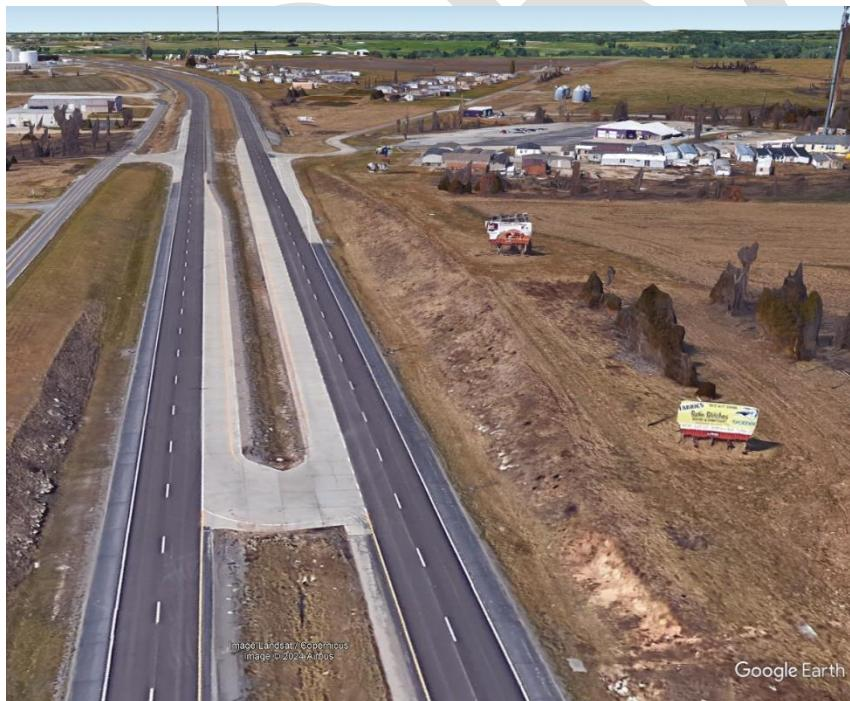
J-turn intersections, also referred to as Restricted Crossing U-turns (RCUTs), are a traffic control design that improves safety and traffic flow by modifying how left-turn and through movements occur at intersections. In a J-turn design, vehicles on the minor road are directed to turn right onto the major road and then make a U-turn at a designated location to continue in their intended direction. This reduces conflict points, significantly lowering the likelihood of severe crashes.
