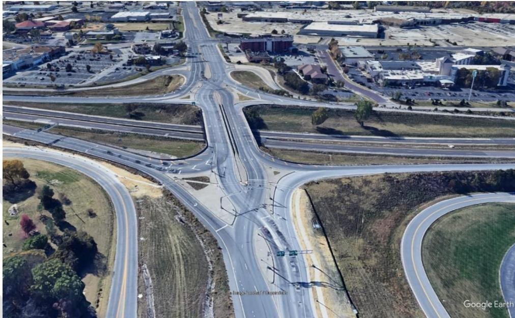
The diverging diamond design is also recognized for its ability to improve safety outcomes. By reducing the number of conflict points and encouraging lower speeds, DDIs reduce the likelihood of high-severity collisions, such as head-on or left-turn crashes. Since its implementation at Stadium Blvd, the intersection has seen improvements in traffic safety, with fewer reported accidents compared to traditional interchanges.
