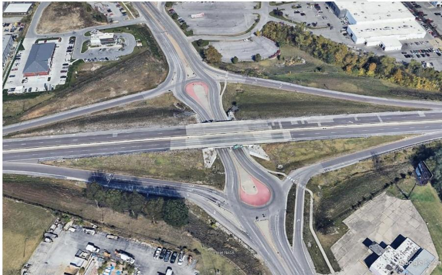
Roundabout interchanges are a modern solution to managing traffic flow and safety at freeway interchanges, offering alternatives to traditional signalized designs. The MPA includes variations of two such interchanges: at I-70 and Business Loop 70, and at I-70 and Rangeline Street. These represent innovative approaches to traffic management, particularly in regions with growing traffic demands.
