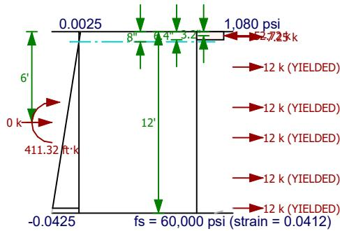
From the analysis, strain in extreme tension bar is 0.0412.
