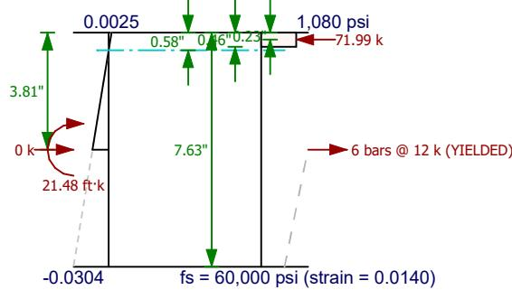
From the analysis, strain in extreme tension bar is 0.0140.
