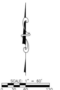
BEARINGS ARE REFERENCED TO GRID NORTH OF THE MISSOURI STATE PLANE COORDINATE SYSTEM NAD83(2011), EPOCH DATE 2010.00, CENTRAL ZONE, BY GPS OBSERVATIONS, USING MODOT VRS NETWORK
