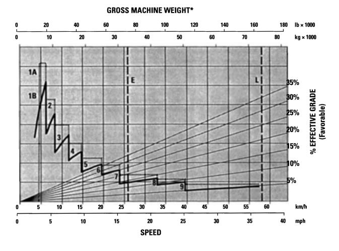
1A – 1st Gear (Converter Drive)
