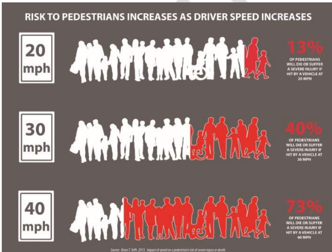
Figure 12: Pedestrian survival rates by vehicle speed 86
