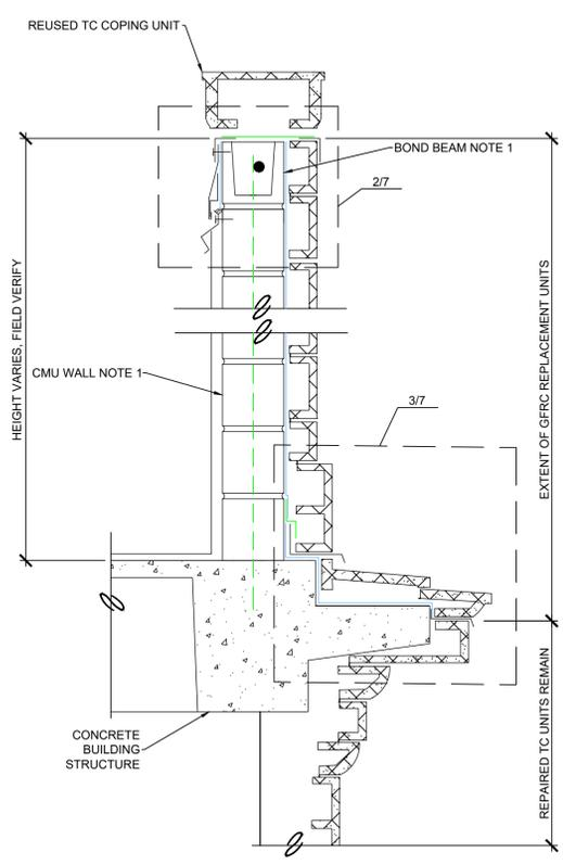
**SCHEMATIC SECTION THROUGH SOUTH PARAPET WALL** 1/7
