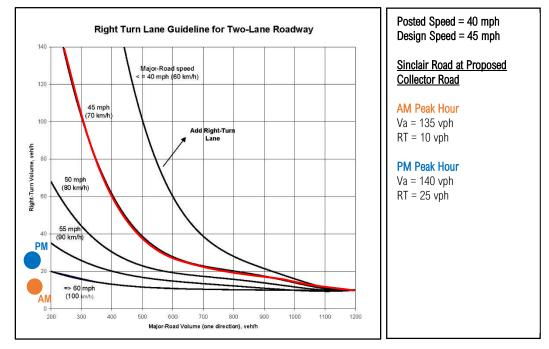
Figure 15: Southbound Sinclair Road Right-Turn Warrants – 2021 Build Proposed Collector Road
