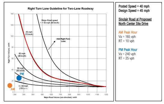
Figure 13: Southbound Sinclair Road Right-Turn Warrants - 2021 Build Proposed North Center Site Drive
