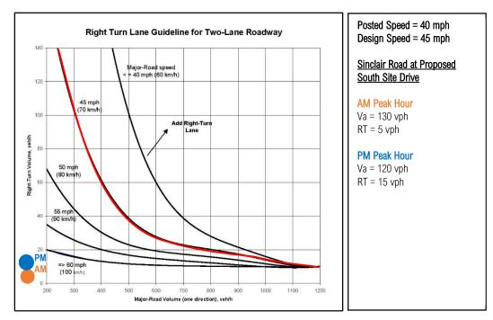
Figure 16: Southbound Sinclair Road Right-Turn Warrants – 2021 Build Proposed South Site Drive
