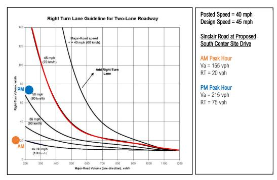
Figure 14: Southbound Sinclair Road Right-Turn Warrants – 2021 Build Proposed South Center Site Drive
