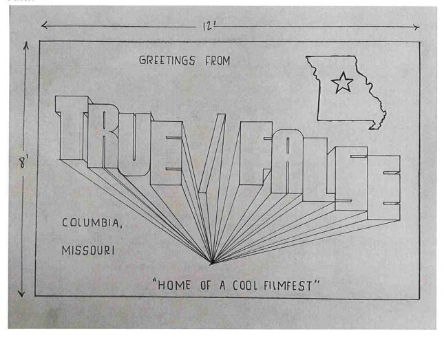
Construction: 8' x 12' (3 panels are 4' x 8') made from reusable, lightweight luan, covered in exterior paint, collage on top, weather proofed with a polyurethane anchored into the wall.
