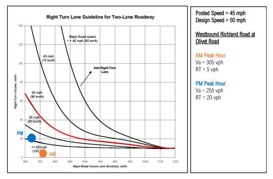
Figure 27: Westbound Richland Road Right-Turn Warrant at Olivet Road – 2021 Build Osburn Farm Alternate
