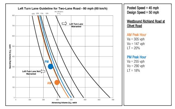
Figure 24: Westbound Richland Road Left-Turn Warrant at Olivet Road – 2021 Build Osburn Farm Alternate
