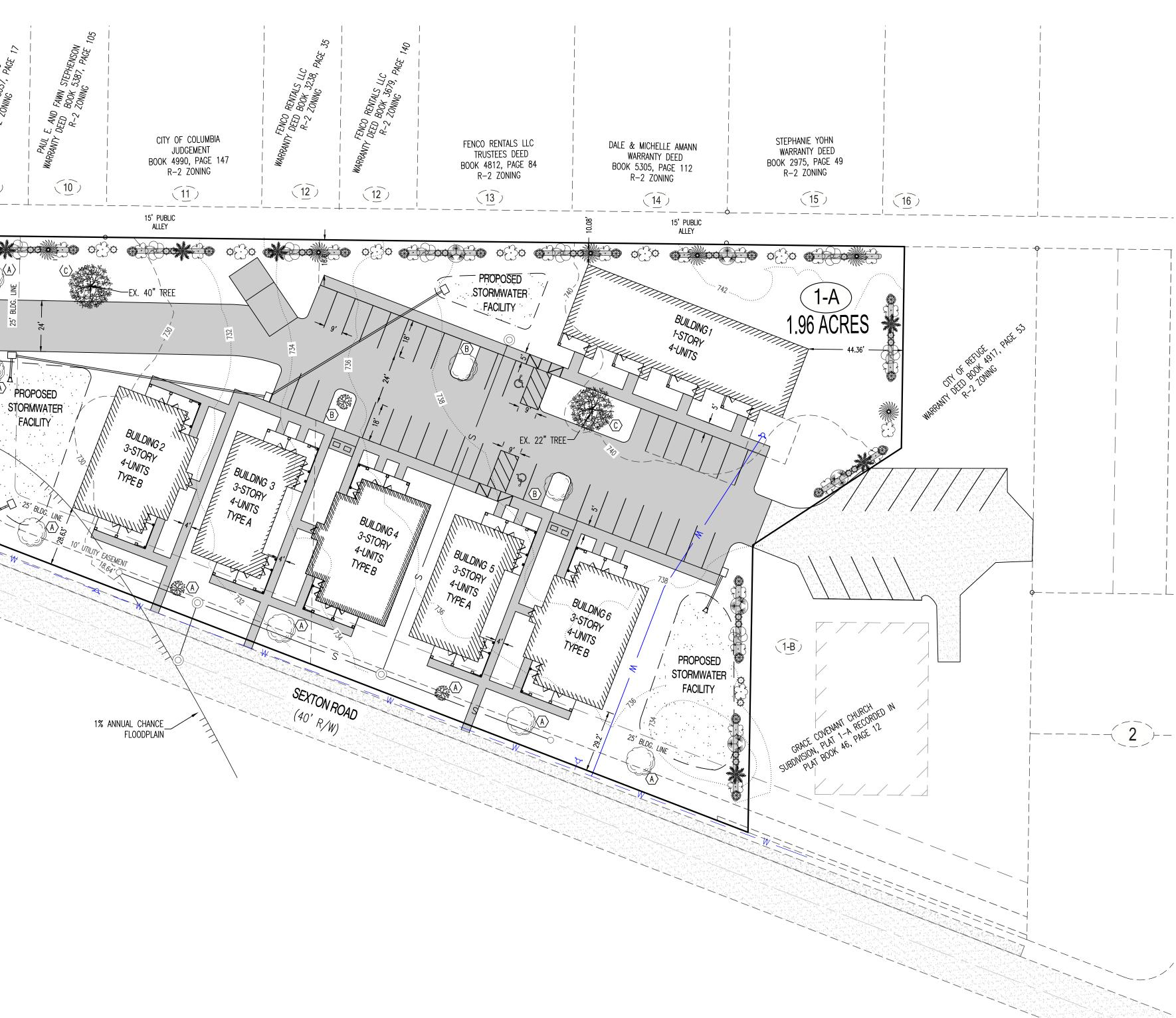
1. 1. ALL DISTURBED AREAS SHALL BE SEEDED & MULCHED AFTER CONSTRUCTION. 2. 2. LANDSCAPING MAY BE ENHANCED BY THE DEVELOPER AS TIME AND BUDGET
